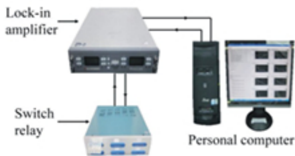
Figure 2. A schematic of the integration of the ESI system.
