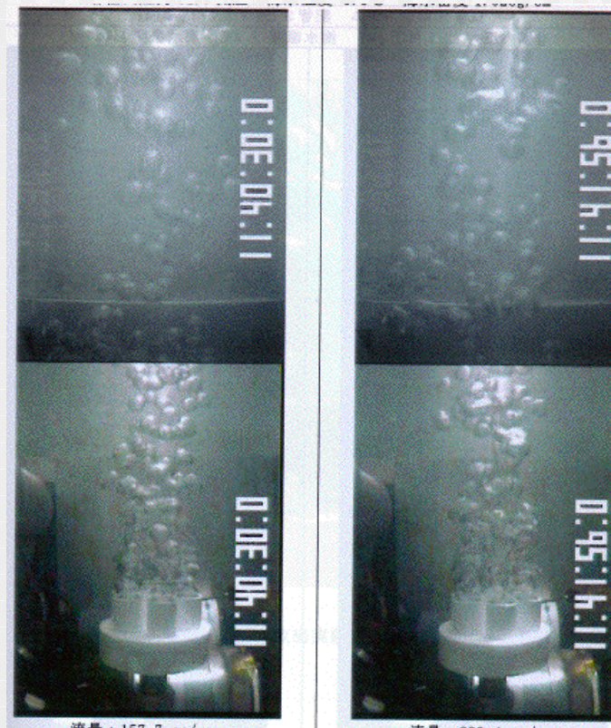
Test of the transport property of the liquid CO 2 (depth 800 m, 3.3° C)
