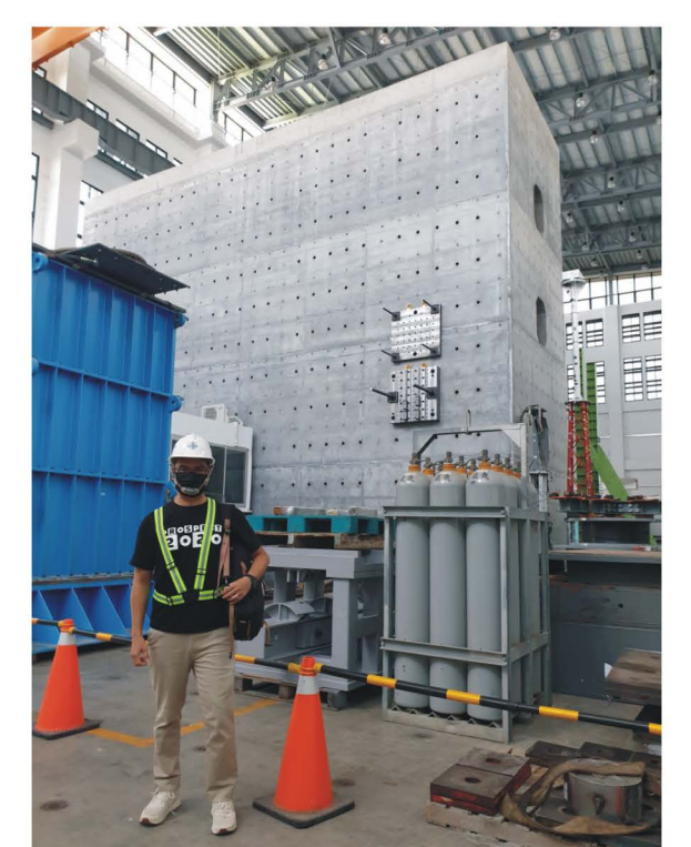
Fig. 3 Strong wall at National Center for Research on Earthquake Engineering (NCEE)
