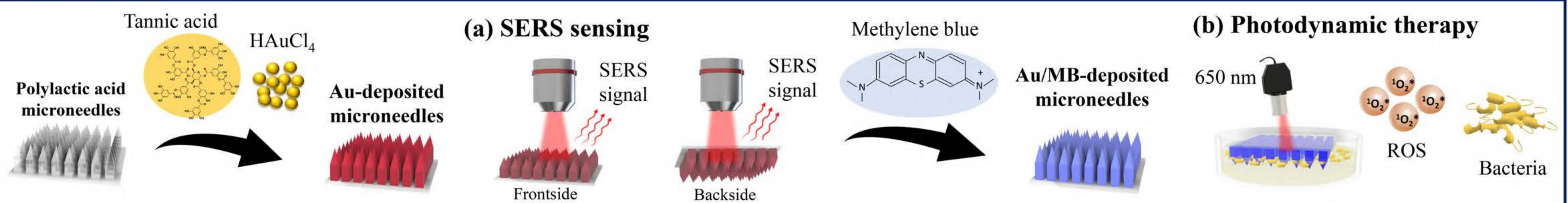
Fig 1. The preparation process of 3D SERS/PDT-active microneedles: Transparent polylactic acid microneedles (PLA MNs) are added tannic acid and HAuCl 4 , forming (a) Au-deposited microneedles (AuMNs) for frontside/backside SERS detection, and subsequently coating with methylene blue to form (b) Au/MB-deposited microneedles (AuMNs-MB) for antibacterial photodynamic therapy.
